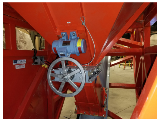
Rotary Electric Vibrator in use above a manual flow gate to rid the hopper of ratholed or hung up material.
