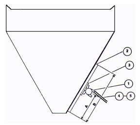
A = 1/3 of the length of the slope portion of the hopper.
