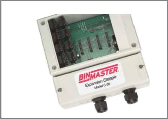
**Lower compartment features** standard size cord grips for power and communications wiring
