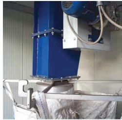
VDC Double Dump Valves are the ideal solution for controlled discharging of powders or granular materials. They are mainly suitable for de-dusting and heavy-duty applications in virtually all industrial sectors. Designed for operating requirements such as high temperatures, highly abrasive materials and/or materials with large grain size. They are also suitable for integration into that do not require continuous material flow.
