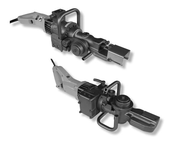
Please note: *This tool is rated for #5 (16mm) Grade 60 Rebar Only*. Do not try to bend or cut material larger in size or rebar harder than grade 60 or you will cause tool damage or machine failure.
