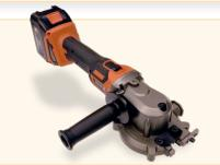
BNCE-20-24V Cutting Edge Saw<sup>™</sup> This is a 24V battery-operated multipurpose cutting tool. Like the corded model above, it can easily cut #6 (3/4") rebar, all-thread rod, chain, EMT conduit, copper pipe, steel rods, steel tubing, and much more. It also features a three position handle. The capacity of the opening is .875" (23.62mm). This tool comes complete with two (2) Li-Ion batteries and charger.
