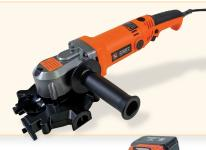
BNCE-30 Cutting Edge Saw<sup>™</sup> A multipurpose cutting tool. It can easily cut #8 (1") rebar, all-thread rod, chain, EMT conduit, copper pipe, steel rods, steel tubing, and much more. This AC powered hand-held tool is lightweight and features a three position handle. The capacity of the opening is 1.18" (30mm). This tool is ETL Listed and is excellent for cutting rebar near flush with concrete or block construction.
