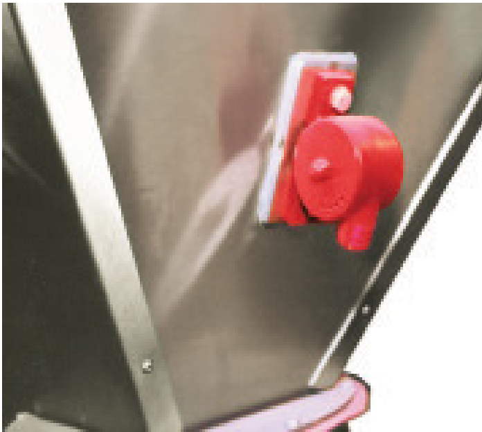
Syntron Pneumatic Turbine Vibrator mounted on stainless steel hopper.
