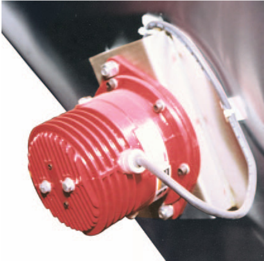
Model V-41 Electromagnetic Vibrator installed on a stainless steel bin.
