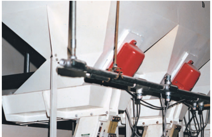
Model V-20 Electromagnetic Vibrators maintain the flow of pasta from bins to packaging lines.
