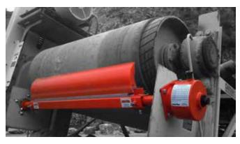
exhibit accelerated wear, discoloration marks, and belt particles baked on the blade. Low tension causes rapid wear because it forces carryback material to pass between the blade and belt at high velocity. This creates channels of uneven wear on the face of the blade. A jagged edge with wear lines on the wear surface indicates a lack of tension. If a cleaner blade's surface is damaged it can no longer conform to the belt's surface for proper cleaning.
