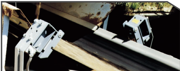
Shown are two BA units protecting a valuable conveyor belt from damage due to belt misalignment or run-off at an aggregate facility.
