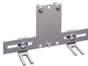
RS-30 BRACKET for mounting the Model RSB stop switch to the conveyor stringer at an idler.
