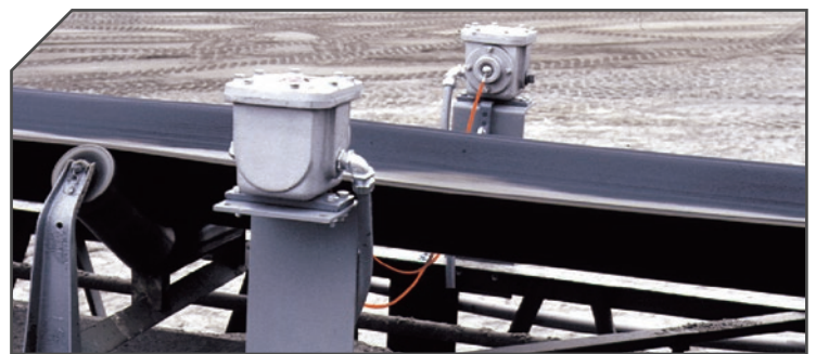
CROSS-SECTION OF CONVEYOR BELT SHOWING INSTALLATION OF UNITS AND CABLE
