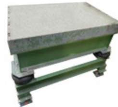
Magnetic Tops for Securing Molds
